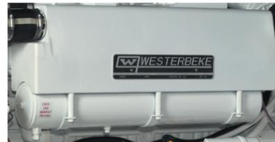
Century Series generators are fresh water cooled with a standard cupro-nickel heat exchanger that mounts directly to the underside of the water-jacketed exhaust manifold for more efficient cooling. This unique Westerbeke design and the use of cast aluminum piping minimizes the use of hose connections in the cooling system, providing added reliability and reduced maintenance.
